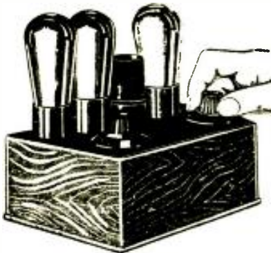
The Model PR-3FS Short-Wave Converter that is, in fact, an all-wave converter, as it enables also the reception of broadcast frequencies. The range is 25 to 600 meters, so you are sure to cover the television band, too.
