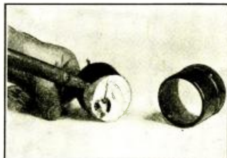
A voltmeter, with its case removed, undergoing the operation described by Mr. Nothelfer, which gives access to the basic milliammeter unit.
